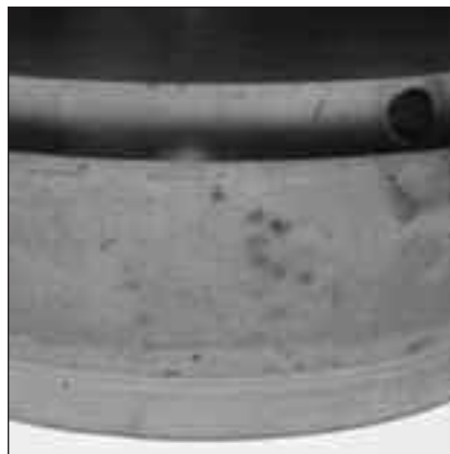
Fig. 21: Peeling on the race of this spherical plain bearing was caused by thin lubricant film.
