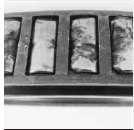
Fig. 29: A heavily overloaded tapered roller bearing resulted in premature, severe fatigue spalling on the rollers. The load was so heavy that large pieces of metal broke off the rollers.
