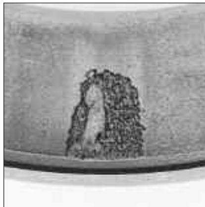
Fig. 54: Localized spalling on this cup race was the result of a stress riser created by a split housing pinch point.
