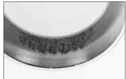
Fig. 36: This irregular roller path is 180 degrees opposite of Fig. 35.
