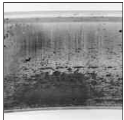
Fig. 22: Micro-spalling or peeling was the result of thin lubricant film from high loads/low RPM or elevated temperatures.
