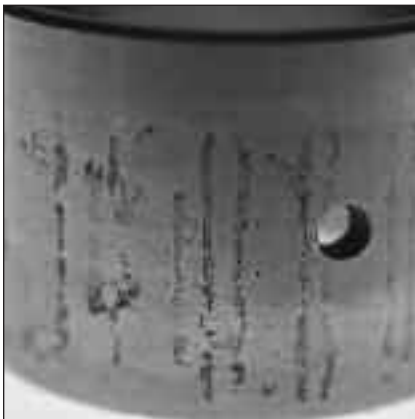
Fig. 12: This cylindrical bearing inner ring has etching and corrosion.
