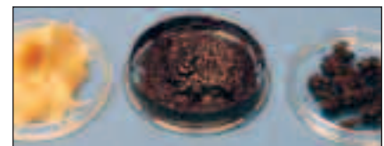
Fig. 87: The above photo shows the same grease at three stages (from left to right): 1) new grease, 2) heavily oxidized grease, and 3) worn-out (failed) grease where the thickener and additives have decomposed and the oil has broken down.
