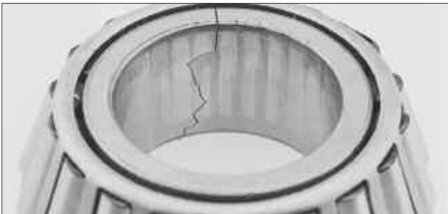
Fig. 58: An out-of-round or oversized shaft caused this fracture on a tapered roller bearing cone.
