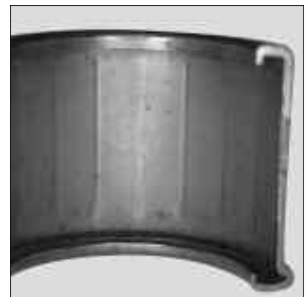
Fig. 62: Impact during installation caused roller spaced indents on this needle roller bearing outer ring.
