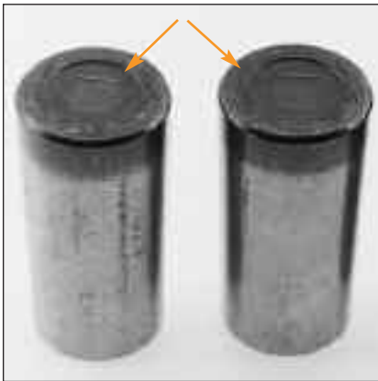
Fig. 17: Heat damage on these tapered rollers was caused by metal-to-metal contact.
