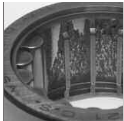
Fig. 38: The housing bore was machined with an improper taper, causing the uneven load distribution and GSC spalling in this cylindrical roller bearing outer ring.
