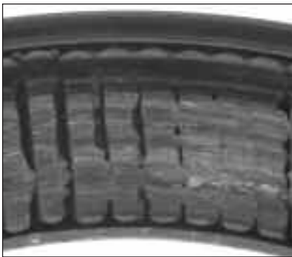
Fig. 74: When the bearing was installed using a pusher without a ball detent to align the rollers, the rollers locked in place as the cup shrunk during installation. The shaft then spun against the locked rollers. (See Fig. 75 right.)
