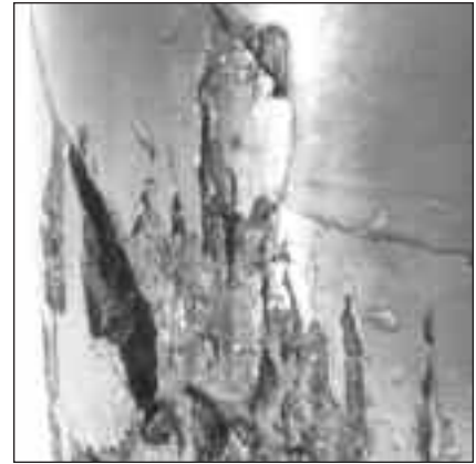
Fig. 24: Heavy spalling and fracturing from high loads on this spherical roller bearing are shown here.
