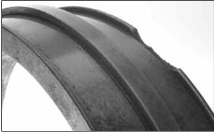
Fig. 40: This spherical roller bearing inner race depicts a fractured toe flange caused by the use of improper installation tools.
