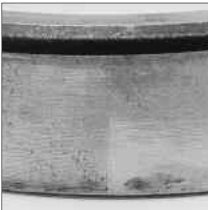
Fig. 53: The marks on the outside diameter of this cup are caused by a high spot on the housing. The cup race is spalled at the spot that corresponds to the spot on the outside of the cup marked from heavy contact.
