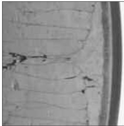
Fig. 61: This cylindrical roller bearing inner ring is crushed by an application failure during service.
