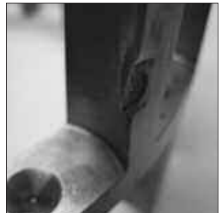
Fig. 49: Poor handling practices caused a deep dent on this spherical roller bearing cage bridge. This damage will result in a lack of proper roller rotation, possible roller skidding, increased temperatures and decreased life.
