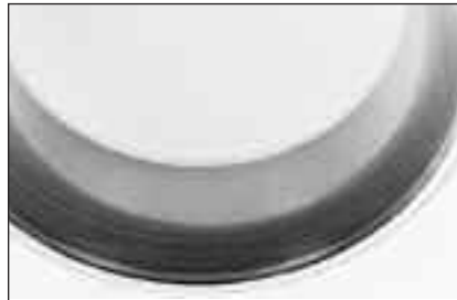
Fig. 35: Deflection, inaccurate machining or wear of bearing seats caused an irregular roller path on this tapered roller bearing outer ring.
