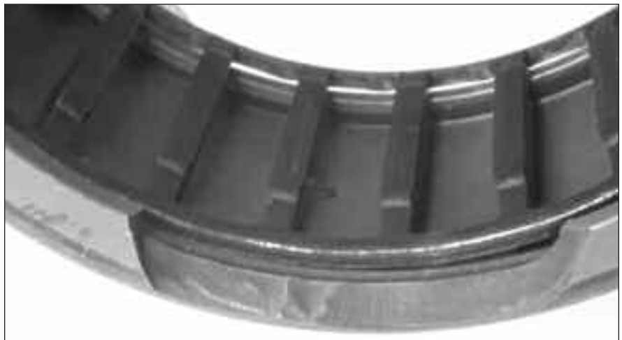
Fig. 42: A hardened driver caused a broken rib on this needle roller bearing.
