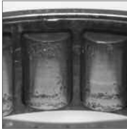
Fig. 23: High loads resulted in fatigue spalling on this cylindrical roller bearing.
