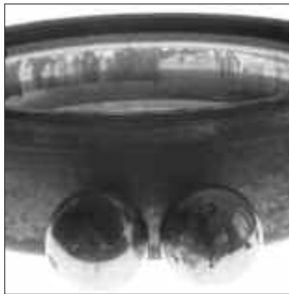
Fig. 16: This ball bearing outer race also depicts etching and corrosion.
