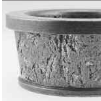
Fig. 30: High loads and low speeds caused insufficient lubricant film on this tapered roller bearing cone.
