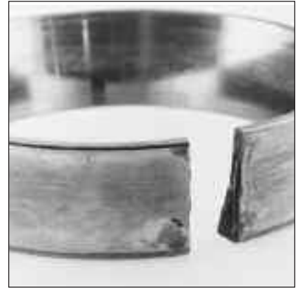
Fig. 56: This tapered roller bearing cup is fractured as a result of the housing cracking during service.
