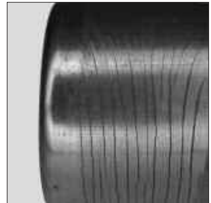
Fig. 73: Very high loading resulted in outer ring sub case fracture of this needle roller bearing.
