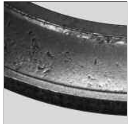
Fig. 32: High load and low speed conditions caused severe peeling and wear on this needle thrust race.
