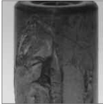
Fig. 28: Overloading on this cylindrical roller bearing caused roller surfaces to fracture.
