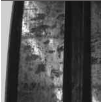
Fig. 50: A worn-out housing caused this bearing to lose fit and fret (move) during service. As a result, metal tearing and wear on this spherical outer ring occurred.
