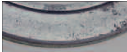
Fig. 83: Peeling (micro-spalling) on this needle thrust bearing inner race was due to a thin lubricant film from elevated temperatures.
