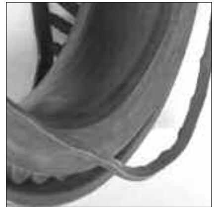
Fig. 19: A misshaped inner ring and torn cage from inadequate lubrication are shown here.
