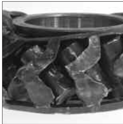
Fig. 18: Total bearing lockup is depicted here.
