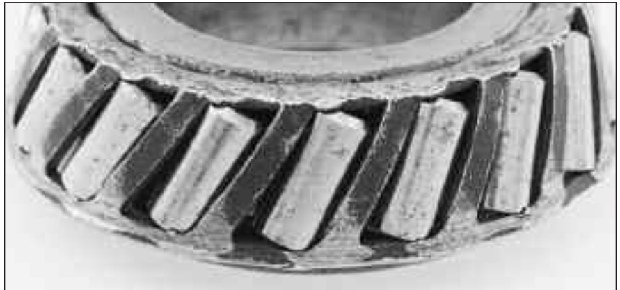
Fig. 47: Binding and skewing of these tapered rollers was due to the compression of the cage ring during installation or interference during service.
