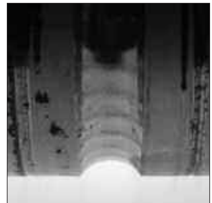
Fig. 64: Shock loading caused brinell damage on this ball bearing inner ring.
