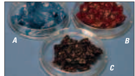
Fig. 85: Grease A and Grease B are not compatible. When mixed together they become lumpy, discolored and hard in composition (Grease C).
