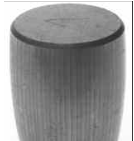
Fig. 68: Welding on a machine, while the bearings were rotating, caused electric arc fluting on this spherical roller bearing.
