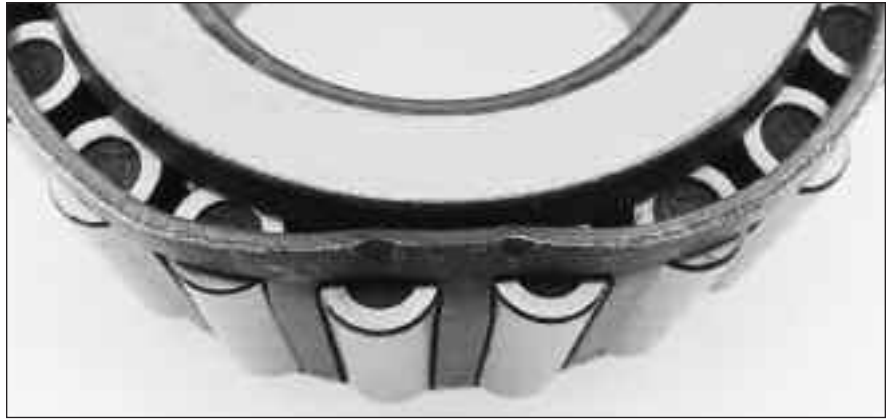
Fig. 46: This cage deformation was caused by an improperly installed or dropped bearing.
