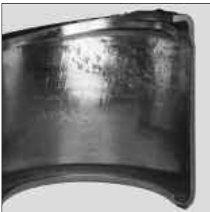
Fig. 71: High loads and extreme misalignment caused roll out of this needle roller bearing outer ring.
