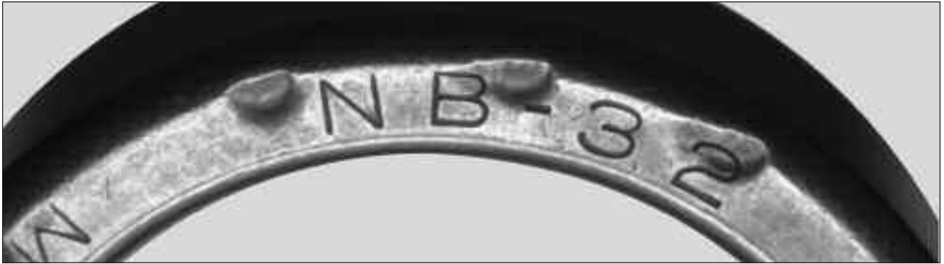
Fig. 43: A hardened punch caused indents during assembly.
