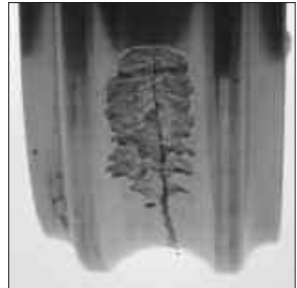
Fig. 26: This ball bearing inner ring depicts fatigue spalling. The fracture is a secondary damage mode.
