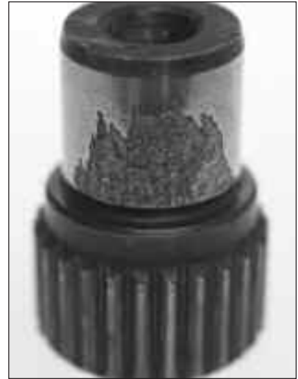
Fig. 33: High edge loads caused Geometric Stress Concentration (GSC) spalling on the inner race of this drawn cup needle bearing.
