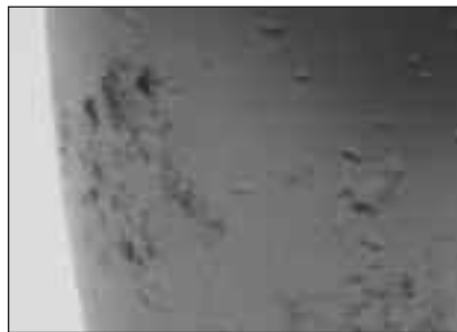
Fig. 8: Hard particles caused contamination bruising on this spherical roller bearing.
