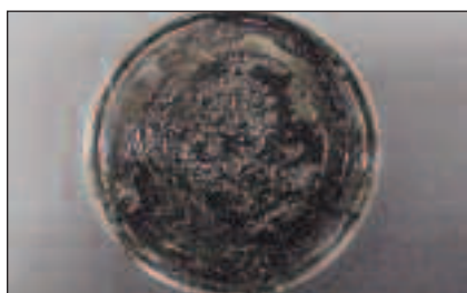
Fig. 79: This petri dish contains heavily oxidized grease, which purged from an overfilled bearing. Grease undergoing heavy oxidation often has a very distinguishable black color and burned odor. In addition, it gets stiffer in consistency.
