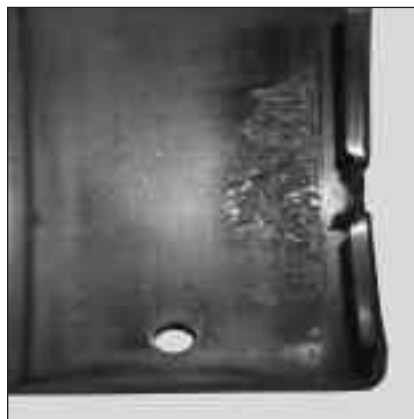
Fig. 37: Geometric Stress Concentration spalling on the outer race was the result of a needle bearing installed in an inaccurately machined housing.
