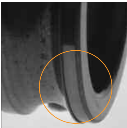
Fig. 20: Excessive heat generation caused metal flow in this ball bearing inner ring.
