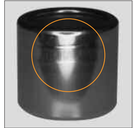
Fig. 52: Inaccurate machining caused a pinch point on this needle roller bearing and grooved the outer ring outside diameter.
