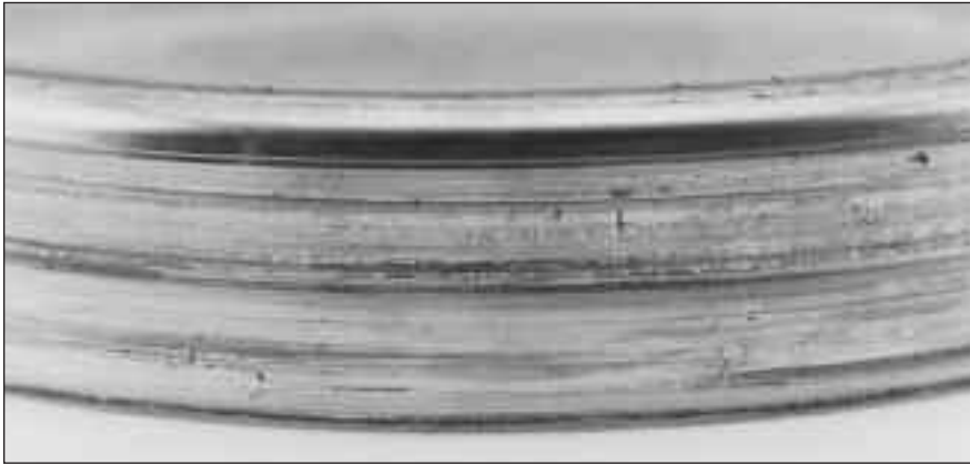
Fig. 55: A loose cup fit in a rotating wheel hub (typically tight) caused this bearing race damage.
