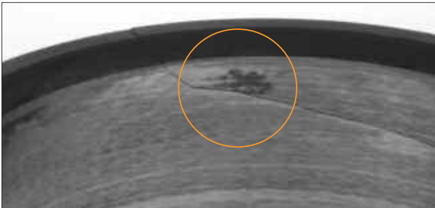
Fig. 57: This ball bearing inner ring fracture is a result of being installed on top of a metal contaminant or raised metal nick.
