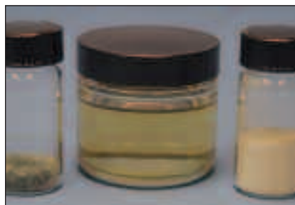
Fig. 86: Grease is a precise combination of additives, oil and thickener.
