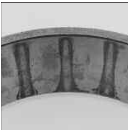
Fig. 15: This cup has heavy corrosion on the race. This type of corrosion may only be a surface stain without pitting. If the staining can be cleaned with a fine emery cloth or crocus cloth, the bearing may be reused. If there are pits that cannot be cleaned with light polishing, the bearing should either be discarded or if practical, refurbished.
