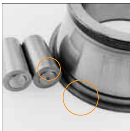
Fig. 3: Fine particle contamination caused abrasive wear on this tapered roller bearing.
