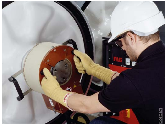
Figure 11 Dismounting of bearing inner rings of wheelset bearings (rail vehicles) using rigid inductor
