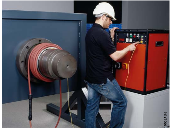
Figure 10 Dismounting of bearing inner rings using flexible inductor
