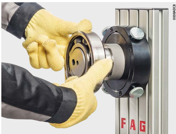
Figure 14 Sliding into place of heated bearing parts
