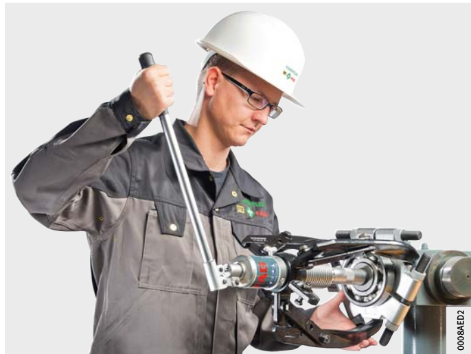
Figure 1 Dismounting by means of extraction device
