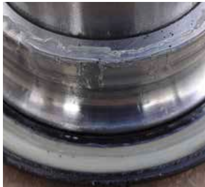
There is no sign of damage or wear to the raceways.
