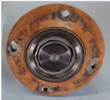
The picture shows that no contamination or rust is present beyond the o-ring.
