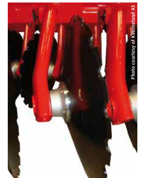
Figure 3: Tested using a water jet for 200 hours. At the end of the test, there was no sign of water having penetrated the cassette seal.
